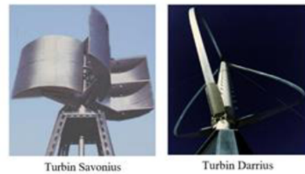
Gambar 1. Tipe turbin angin VAWT (Ambrosio & Marco, 2010)
